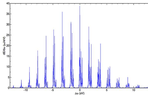
Fig. 5. Spectrum of a mode-locked configuration with module length of 12 undulator periods in the soft-X-ray regime<sup>12</sup>.
