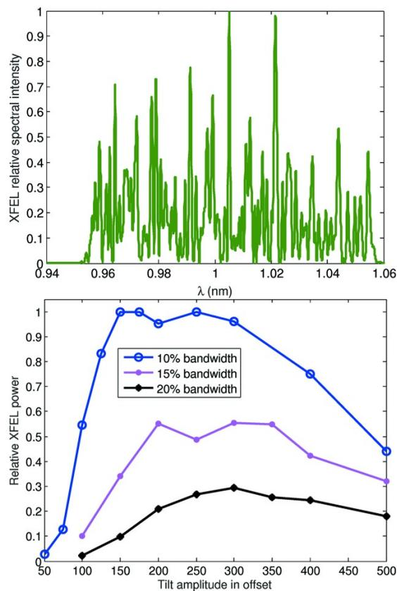
Fig. 4. Simulated spectrum for the SwissFEL soft-X-ray beamline Athos with an injected tilted beam and transverse gradient in the undulator field (upper plot). Optimization of tilt amplitude and gradient for various values of bandwidth in the FEL spectrum<sup>10</sup>.
