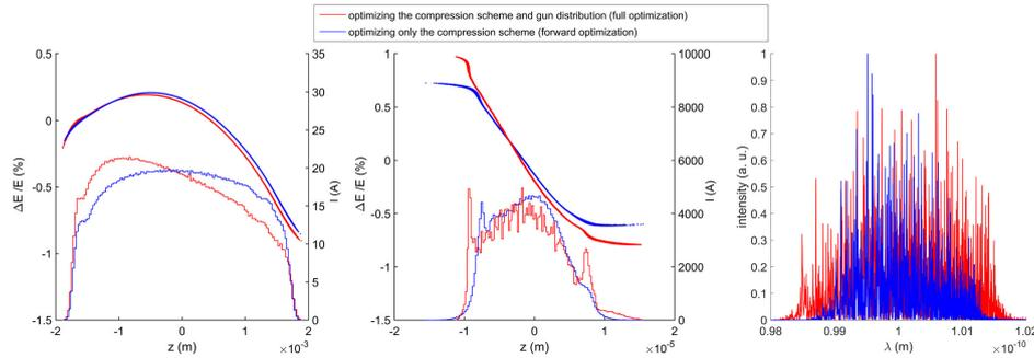
Fig. 2. Simulation for SwissFEL of initial and final current distribution, longitudinal phase space and the corresponding FEL spectrum (left, middle and right plot, respectively), with and without optimizing the laser profile at the cathode<sup>5</sup>.
