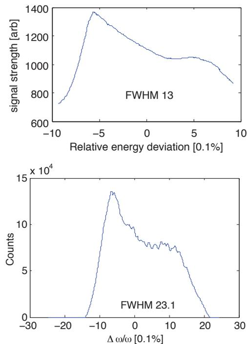
Fig. 1. Energy distribution of the electron bunch and envelope of the FEL spectrum (upper and lower plot, respectively) for an overcompressed bunch at LCLS<sup>2</sup>.
