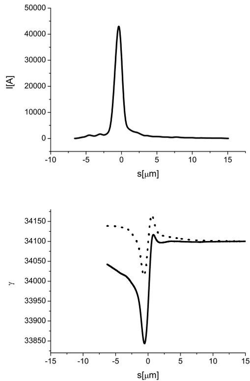
Fig. 3. Simulation for the European XFEL beamline SASE3 for a fully compressed bunch with its current profile and correlated energy distribution (upper and lower plot, respectively)<sup>6</sup>.
